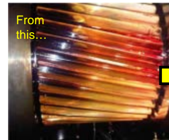
BEFORE (brownish varnish coats the gear)
